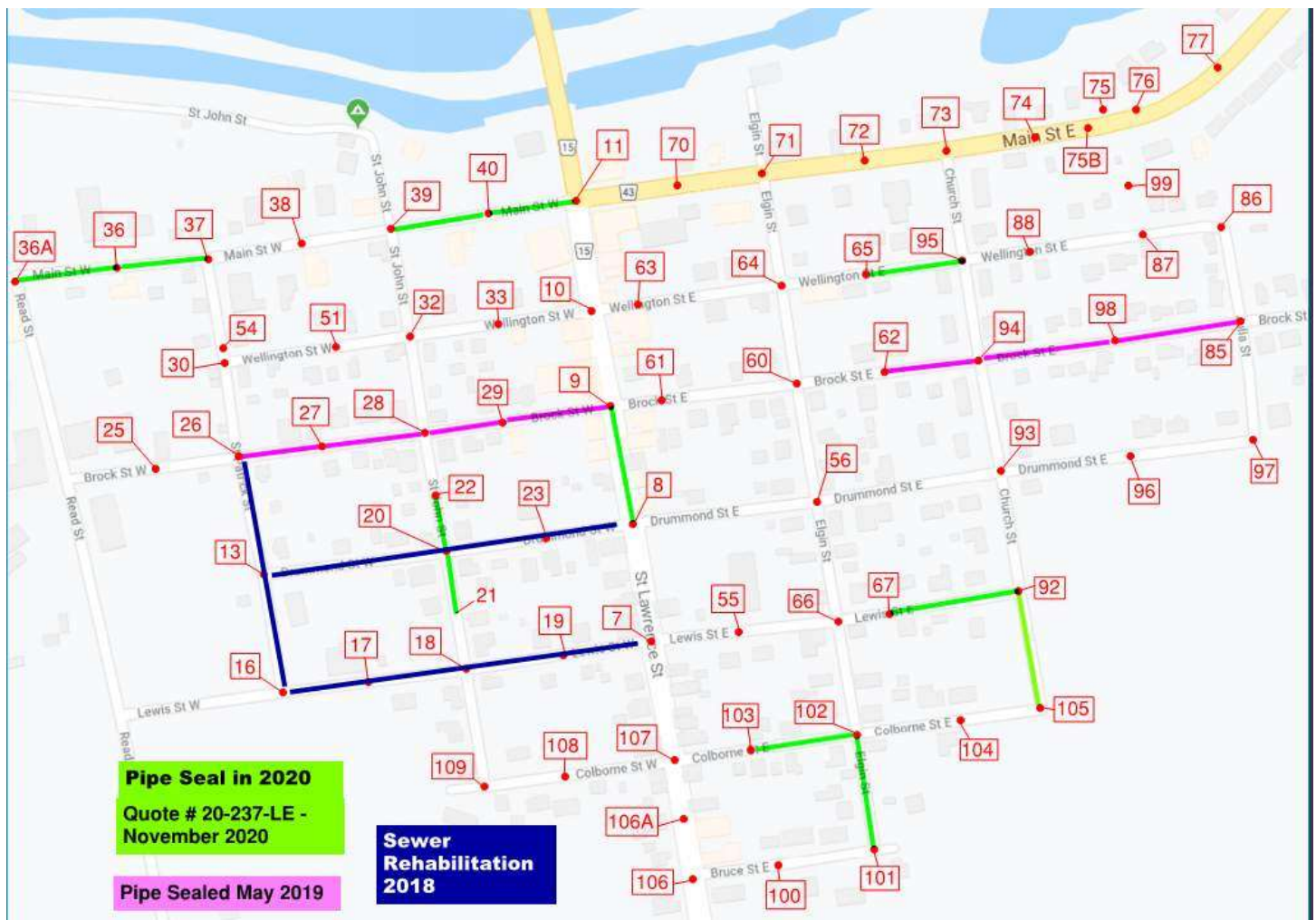
Figure 8: Scope of Sewer Repair Work 2018 - 2020
